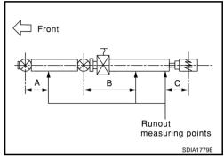
2. If the play exceeds specifications, replace propeller shaft assembly.
