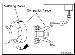
3. If the propeller shaft or final drive has been replaced, connect the propeller shaft and final drive as follows:
