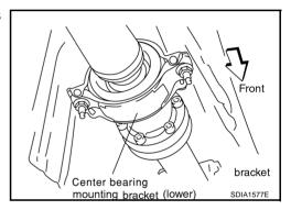
5. Put matching marks on flange and rear propeller shaft.
